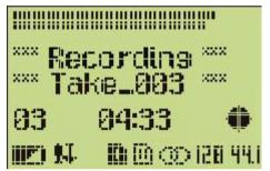
Interrupt the recording temporarily by briefly pressing the PLAY/PAUSE button. Pressing the STOP button will end the recording.
